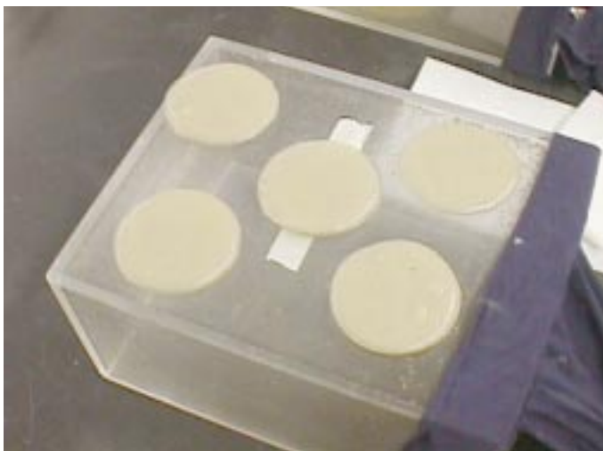
Figure 4. Eggs are from the CU flies on watch glasses with standard food. Each cage receives five watch glasses for 24 hours.
