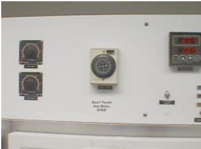
**Figure 1.** The control panel for the large double-door incubators in the Mueller and Rose labs.
