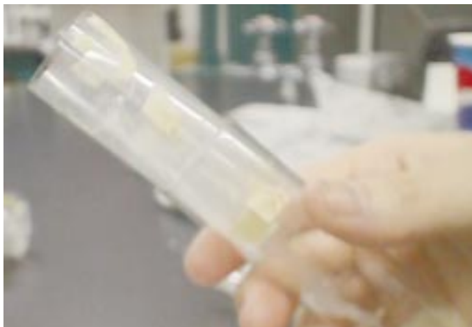
Figure 9. Plastic sleeves are inserted into each vial after eggs have been added. The fit must be tight and the sleeve should be pushed all the way down to the food.
